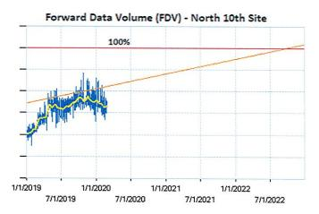
Summary: The existing Auburn and North 10<sup>th</sup> sites will not be able to support the traffic in the area they cover in the future as shown above by the orange trend line meets the red exhaustion threshold. When this occurs 4G data speeds slow to unacceptable levels.
