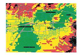
Coverage is best shown via coverage maps. RF engineers use tools that take into account terrain, vegetation, building types, and WCF specifics to model the existing coverage and prediction what we expect to see with the addition of a proposed WCF.
