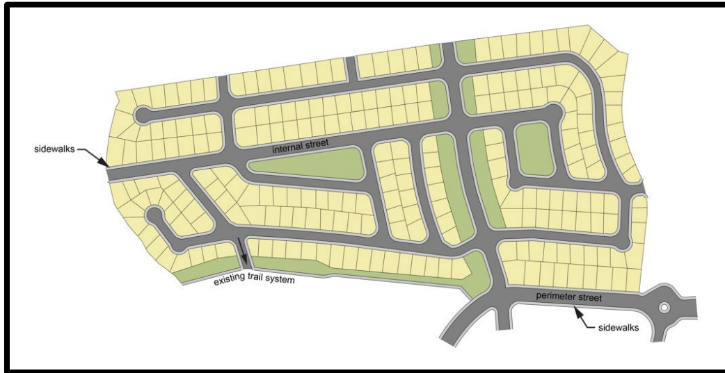
Figure 5.3.8-1: Sidewalk Installation for Multi-Lot Subdivisions
